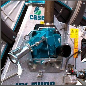
The gear box is directly connected with turbine and ring gear with ultimate technology in order to provide minimum pressure loss and enhanced performance for the hose reel.
